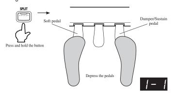
The LED indicator for the SPLIT button will start to flash, indicating that FOUR HANDS mode has been activated.
